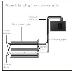
While each sampling method is suited to specific applications, more than one method is often effectively employed to monitor a firezone. In some applications - particularly those in which there is movement of high volumes of air – the most effective sampling network generally combines two methods to provide maximum coverage to a zone under all operating conditions.
