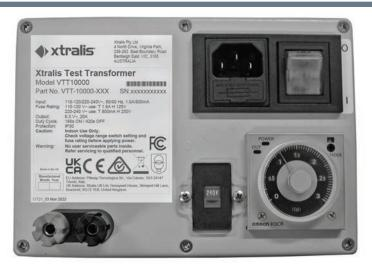
Xtralis Test Transformer VTT-10000 (previously known as the Hot Wire Test – Power Supply Unit (PSU)) is a tool used to test very early warning aspirating smoke detection equipment.
